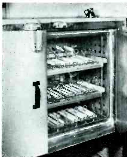
Figure 6. The trays are now transferred to an electric oven and the crystals are baked for several hours. After baking, the crystals are checked for frequency and are then issued to the finishing department where they are individually etched by hand exactly to final frequency.
