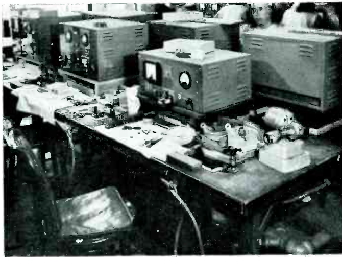
Figure 7. A final finishing position where the crystals are individually etched to the desired final frequency. The crystals are held in plastic tongs and are etched in a dish of Frequency-Etch solution. During the etching the frequency is checked intermittently against the standard frequency in a comparison oscillator until the desired value is reached. The crystal activity is brought up, if necessary, by edge grinding in a Hudson American diamond-Bonded edging wheel (right).
