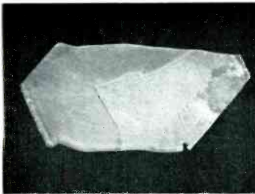
Figure 1. A sawn wafer of quartz in which electrical twinning has been revealed by etching.
